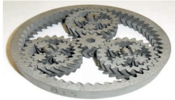
Figure 4: A Complex Gear System Produced Using 3D Printing without supporting assemblies.
